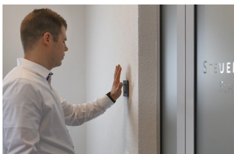
Palm vein scanner- iCognize Manuscan 2
