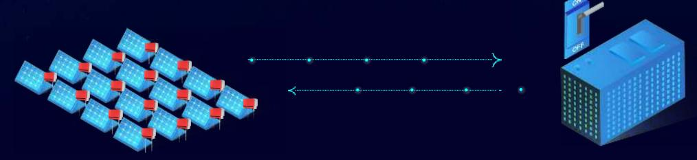
Support up to 40 inverters in series Shut down multiple inverters within 0.2s Emergency Power Off– to turn off all inverters rapidly by remote one-button operation
